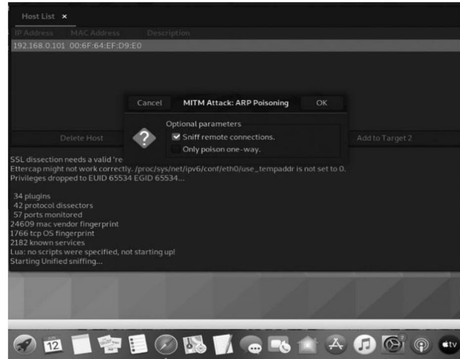
FIGURE 7.9 Unified sniffing on remote connections using MITM attack, using ARP spoofing technique.
